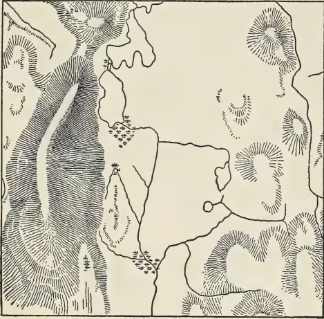
A hachure map uses little lines to show the shape and slope of the land.
